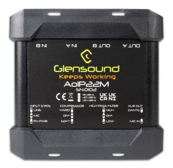
The AoIP22M is digitally controlled. This allows us to have additional functionality that can be easily selected with the front panel switches. The switch function is detailed on the top panel as shown above.
