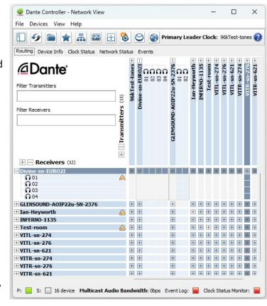
logging, enabling you to quickly identify and resolve any potential network issues. You can also quickly and easily backup, restore, move, and reuse Dante network configurations using Presets, and edit Dante routing configurations offline.
