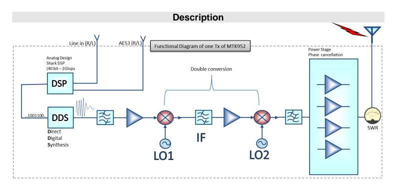
MTK952 is a versatile dual transmitter capable of working in a huge UHF bandwidth and of generating any kind of narrow-band modulations, with very high quality and low spurious emissions.
